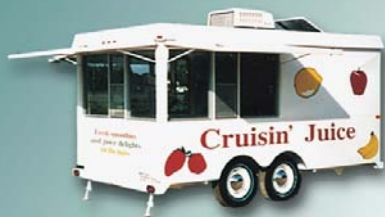
MODEL CF14 14' x 8' with optional California windows, roof vent, air conditioner, water system, refrigerator, ice chest and graphics
